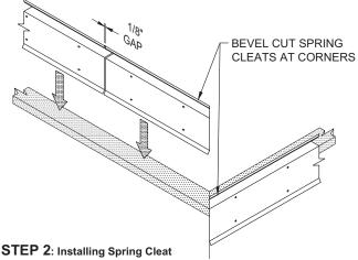
Prior to installing the spring cleat, ensure that all metal components have been isolated from ACQ treated lumber with appropriate membrane material. Field cut spring cleat to fit corner conditions. Install spring cleat working away from corners. Allow 1/8" gap between sections for thermal movement. Attach the spring cleat using the 1-1/2" ss ring shank nails provided in each pre-punched hole.
