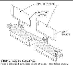
over the top of the spring cleat. Press down on the fascia until the drip edge in engaged. Slide fascia into place.
